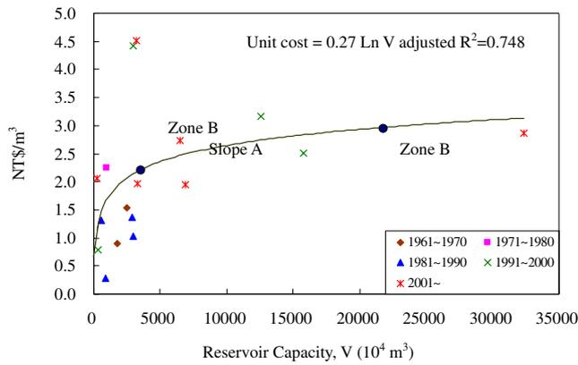
**Fig. 7** Analysis construction costs based on existing and planned reservoirs in Taiwan
