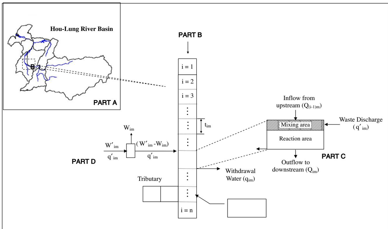
**Fig. 2** The schematic representation of subscripts and parameters used in the model
