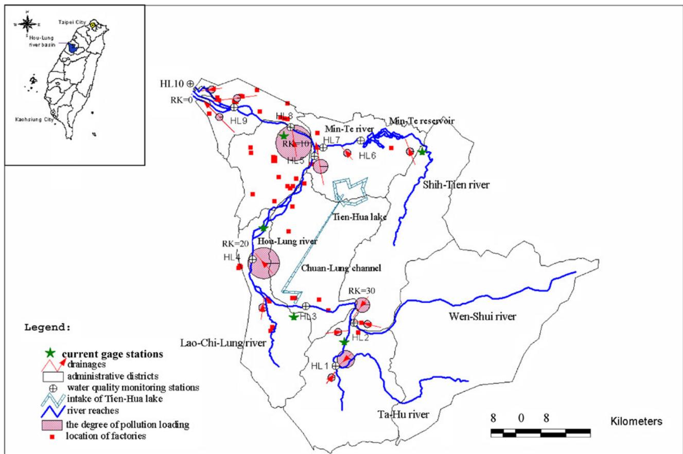
**Fig. 1** Distribution of the waste load and monitoring stations in Hou-Lung River system
